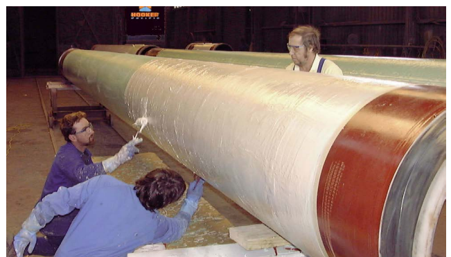
Ceilcote® 242GF Flakeline applied to protect steel pipes used offshore by the Oil & Gas Industry.
