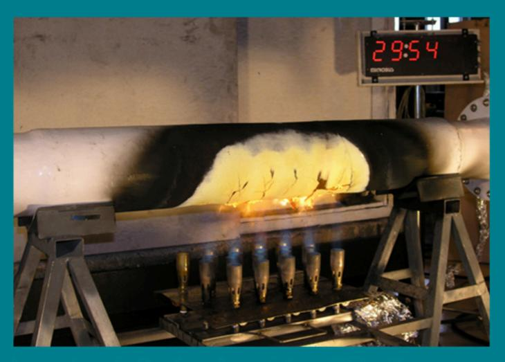
Armatec's standard marine exhaust tubing and WhispaPipe factory insulated marine exhaust tubing have been tested to and passed tests specified by "IMO Resolution A.753(18), Appendix 2". This test requires the water filled pipe to maintain its structural integrity for at least 30 minutes in the event of a fire. The testing institute was SP Fire Technology of Sweden.
