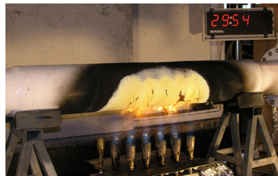
WhispaPipe meets IMO fire endurance tests. Contact ARMATEC or visit website for IMO test certificate.
