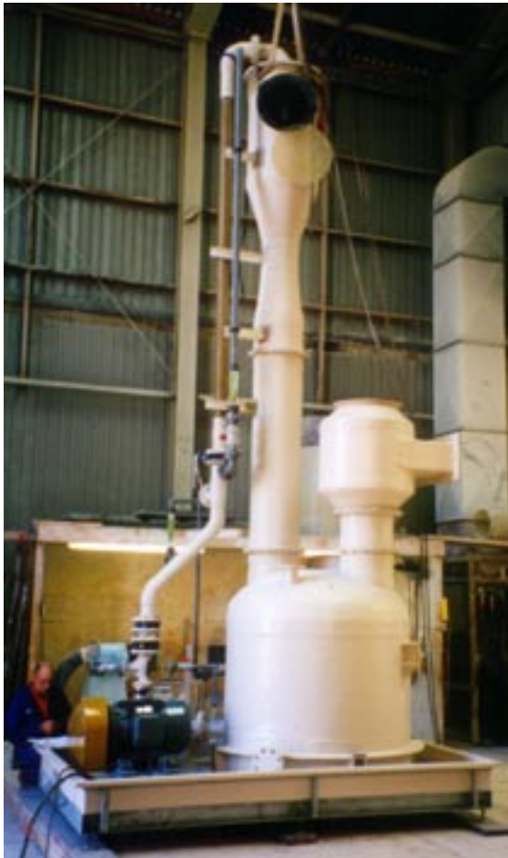
Eductor venturi scrubber for collecting particulate and gaseous pollutants from sulphur melting operation. Unit has mesh pad type mist eliminator.
