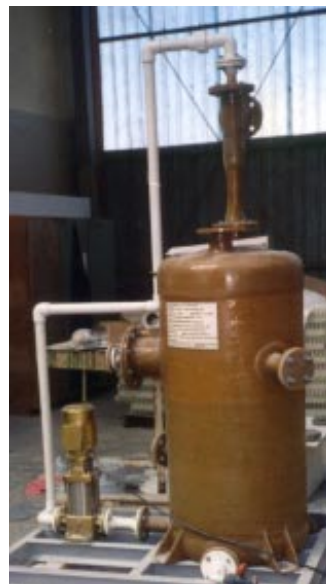
Small eductor venturi scrubber for collecting cyanide dust from bag opening operation.
