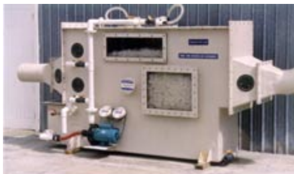
ARMATEC's pilot plant crossflow scrubber. Capacity 1m 3 /s.
