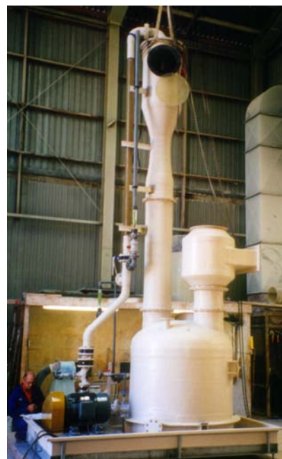
Above: Multi-throat venturi scrubber removing particulate from vents from food processing operations. Right: Eductor venturi for collecting toxic dust.
