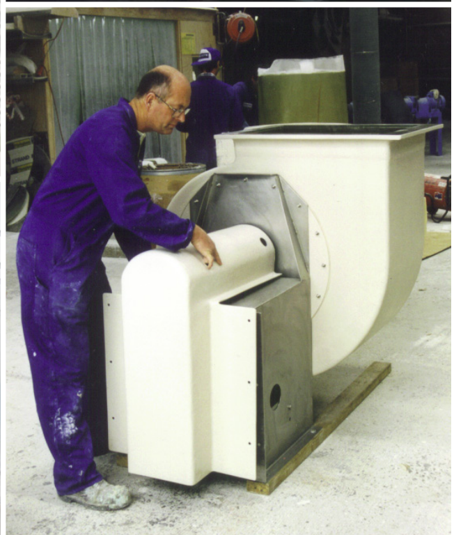
Left: Axial fans, duty and standby, providing fresh air to biosolids processing building at WWTP. Right: Large and small centrifugal fans being assembled ready for despatch.
