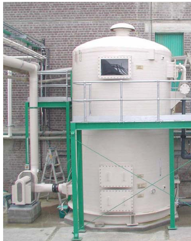
Biological scrubber removing H 2 S from gas stream ex sulphur melter at fertiliser plant.
