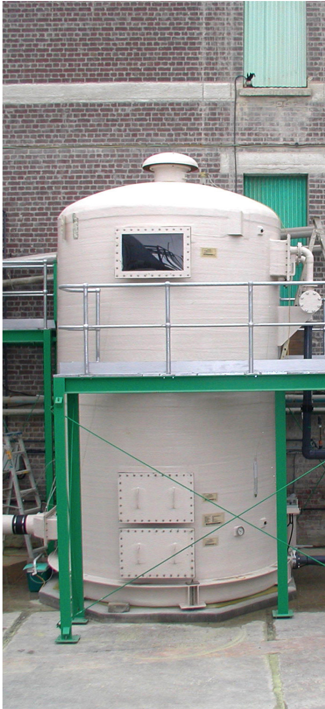
Left: Biological scrubber removing H_2S . Top right: Biological scrubber pilot plant at pump station. Bottom right: ARMATEC designed biological scrubber at Sydney WWTP.
