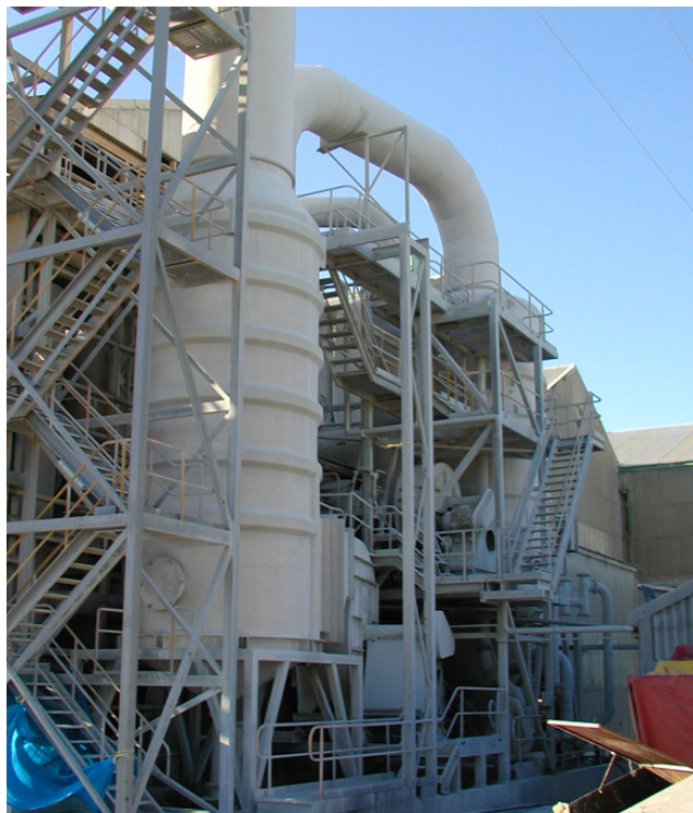
Left: Wet cyclone at fertiliser plant, for removing liquid droplets after void tower scrubbers. Right: Kimre mist eliminator removing acid droplets and water mist from air stream.
