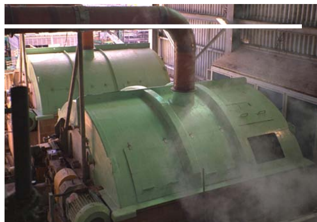
Top left and right: Removeable segmented covers over inlet chambers and PST tanks at wastewater treatment plant. Bottom left: Removeable cover over tank at wastewater treatment plant. Bottom right: Covers over pulp washers at pulp and paper mill.
