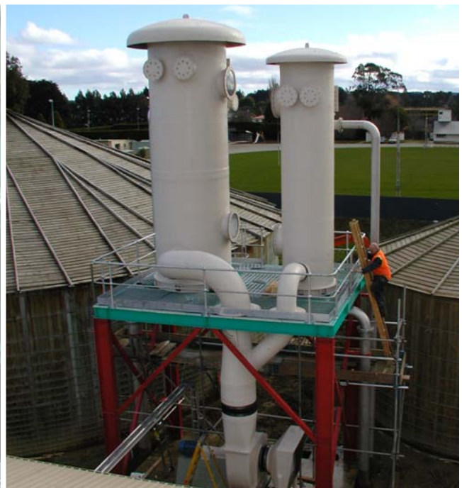
Left: Cyclones at two fertiliser plants, last stage of mist elimination before discharge to stack. Right top: Kimre mist eliminator for acid mist collection at battery plant. Right bottom: Gas strippers removing carbon dioxide from water.
