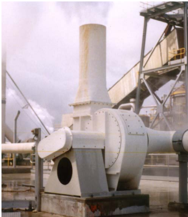
Left: Centrifugal fans installed at fertiliser plant (top), and pulp and paper mill (bottom).
