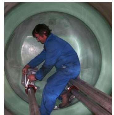
Nozzles, ladders, pump guide rails and discharge pipes are all factory fitted.
