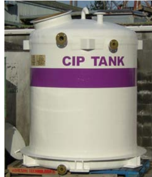
Fibreglass tank for CIP wastewater
