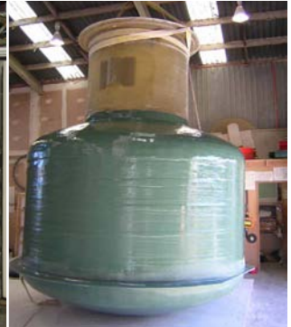
Pump station with extra storage capacity
