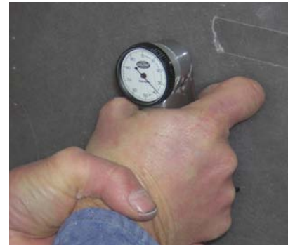
Barcol Hardness testing to check laminate is cured
