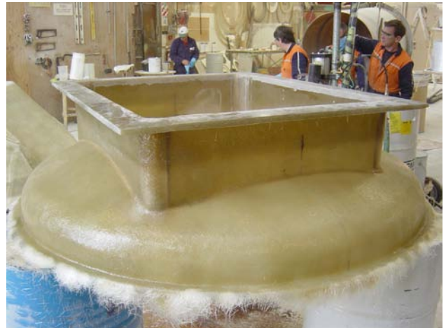
Fibreglass pump stations parts are all manufactured and assembled in ARMATEC's factory.
