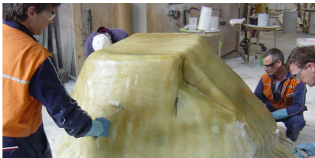
Flygt TOPS bases are used to optimise hydraulics and minimise liquid retention. All joints are butt and strap jointed outside and inside to create a liquid tight envelope that cannot leak.
