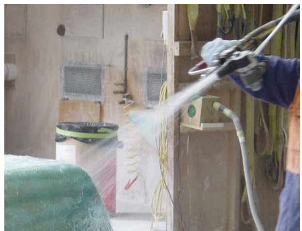
Chopper gun simultaneously applying chopped glass fibre and resin to a mould.
