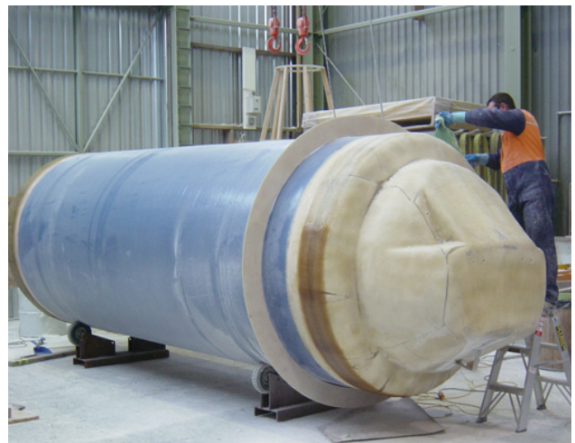
Flygt TOPS bases are used to optimise hydraulics and minimise liquid retention. All joints are butt and strap jointed outside and inside to create a liquid tight envelope that cannot leak.
